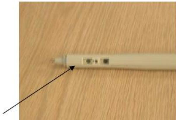
4. Pull the inner housing from inside the shell by pulling on the power cord. This may require force because the PCB is soldered to the inner housing and the shield, which lines the outer shell.
