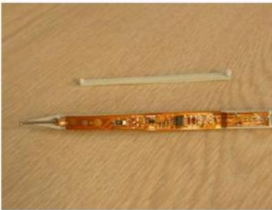
8. Pull the power cord, which is soldered to the PCB, out of the inner housing.
