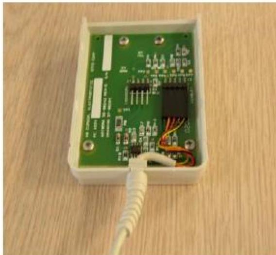
5. Unscrew the PCB and remove it from the inner housing.
